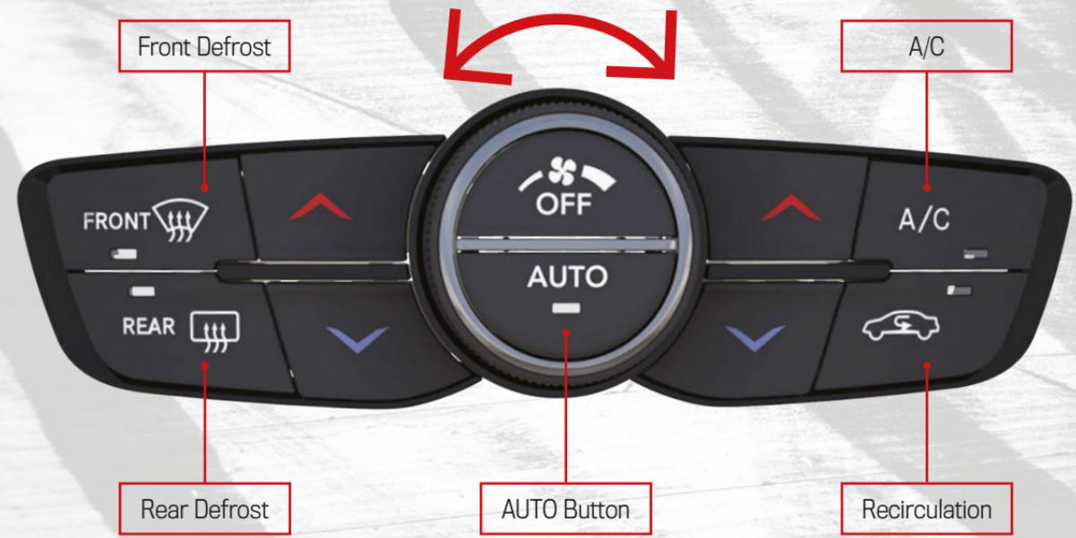
**TIP:** Push the **red** arrow button to increase the temperature or push the **blue** arrow button to decrease the temperature for the driver or the passenger.
