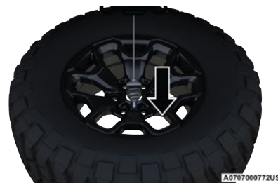
Positioning Retainer Through Center Of Wheel
