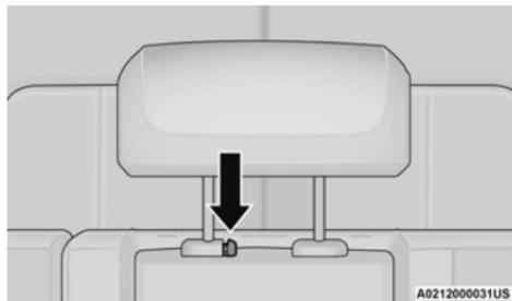
Center Seat Head Restraint Adjustment Button
