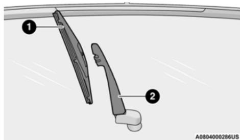
**Wiper Blade Removed From Wiper Arm**
