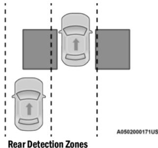
When the vehicle is started, the BSM Warning Light will momentarily illuminate in both outside rearview mirrors to let the driver know that the system is operational. The BSM system sensors operate when the vehicle is in any forward gear.
