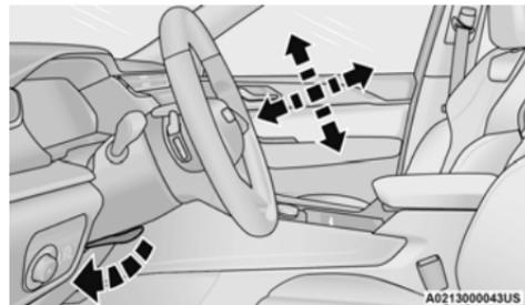
Manual Tilt/Telescoping Steering Column Handle
