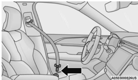
**Inserting Latch Plate Into Buckle**
