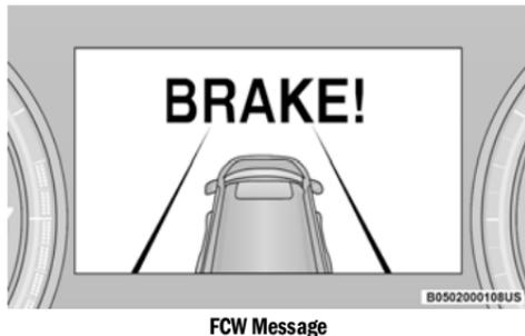
When the system determines a collision with the vehicle in front of you is no longer probable, the warning message will be deactivated [↪ page 344](#).
