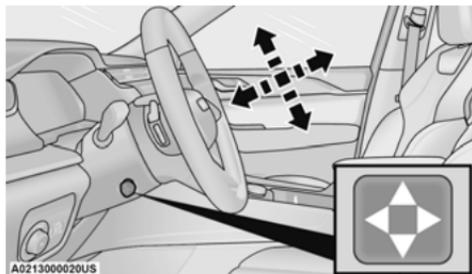
**Power Tilt/Telescoping Steering Control Location**
