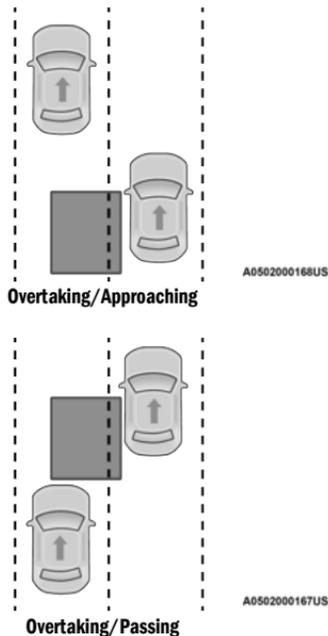
The BSM system is designed not to issue an alert on stationary objects such as guardrails, posts, walls, foliage, berms, etc. However, occasionally the system may alert on such objects. This is normal operation and your vehicle does not require service.
