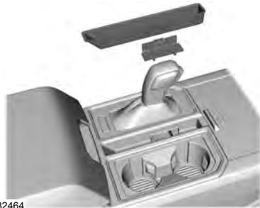
3. Locate the white brake shift interlock lever on the passenger side of the shifter assembly.
