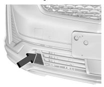
Remove the engine heater connector cover by gently prying with a flat-bladed tool at the location of the notch along the top edge of the cover.
