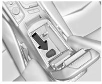
Place the new remote key into the remote key pocket. The remote key pocket is inside the center console storage area between the driver and front passenger seats. The storage area will need to be opened and the storage tray lifted up to access the remote key pocket.
