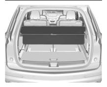
If equipped, the cargo cover is used to cover items in the cargo area. It is foldable and stores in the cargo storage bin under the load floor when not in use.
