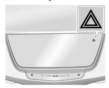
$\triangle$ : Touch  $\triangle$  on the center stack to make the front and rear turn signal lamps flash on and off. Touch again to turn the flashers off.
