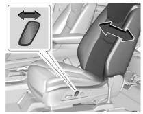
Tilt the top of the control rearward to recline.  Tilt the top of the control forward to raise.
