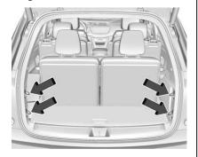
The vehicle has four cargo tie-downs in the rear compartment.
