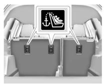
The top tether anchors are on the rear of the seatback for each seating position in the second row.
