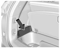
The rear compartment fuse block is in the cargo area, on the driver side of the vehicle behind the lower trim panel. To access the fuses in the Rear Electrical Center, remove the center cargo bin, then small side bin. See *Rear Storage* ⇔ 86. See your dealer if additional assistance is needed.
