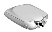
Separate the two halves of the remote key using a flat tool inserted into the bottom center of the remote key. Do not use the key slot.
