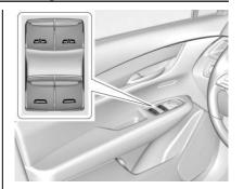
The power windows work when the ignition is on, in accessory mode, or when Retained Accessory Power (RAP) is active. See Retained Accessory Power (RAP) ⇒ 205.
