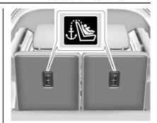
The top tether anchors are on the rear of the seatback for each seating position in the third row.
