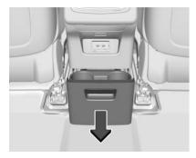
If equipped with cupholders in the back center console, pull on the handle to access.
