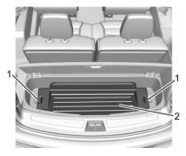
Remove the cargo management system tray (2) by pulling on the handles (1). See Cargo Management System
