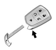
To remove the key, press the button on the side of the remote key, near the bottom, and pull the key out. Never pull the key out without pressing the button.
