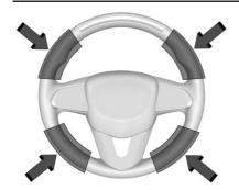
Any time the steering wheel light bar flashes red, resume manual steering immediately. The instrument cluster light ), will also turn red and a message will display in the Driver Information Center (DIC). In addition, beeps will sound, or the Safety Alert Seat will vibrate. To view available settings from the infotainment screen, touch Settings > Vehicle > Collision/Detection Systems. After you begin steering manually, then Super Cruise will disengage.
