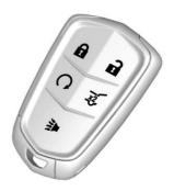
ress to lock all doors and if equipped, the fuel door. The turn signal indicators may flash and/or the horn may sound on the second press to indicate locking. To view available settings for this feature, touch the Settings icon on the infotainment home page. Select "Vehicle" to display the list of available options and select "Remote Lock, Unlock. Start".
