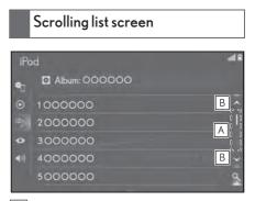
A Select this part to scroll the list by operating the scroll bar. To release scrolling the list, select the scroll bar again.
