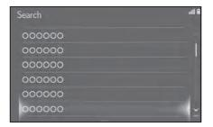
10.3-inch display model: When text is input, a candidate list of items to search for is displayed on the side screen.
