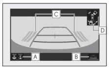
A Display mode switching button Each time the button is selected, the rear view mode and the wide rear view mode
