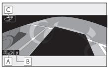
A Display mode switching button Select to change the display mode between the moving view and the see-through view.
