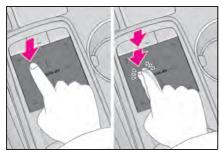
When the pointer moves close to a button, it will automatically snap to that button and the Remote Touch feedback force (vibration) is generated by the touchpad. This feedback force can be adjusted. ( $\rightarrow$ P.70)
