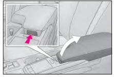
• Lift by hand to fully open the console box.
