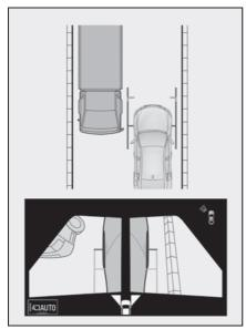
• Check the positions and distance between the vehicle width guide line
