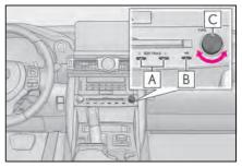
A Press to select a track. Press and hold to fast forward/rewind.
