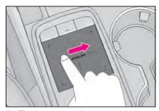
The buttons on the screen can be selected by either depressing or double tapping on the touchpad.
