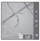
A Select the map to switch it between displaying only the area around the destination and the area from the current location to the destination.
