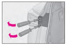
3 Pull the cover toward the rear of the vehicle to remove it.
