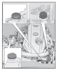
IS500: Do not loosen the coolant inlet cap or coolant reservoir cap while the engine and radiator are hot. High temperature steam or coolant could spray out.
