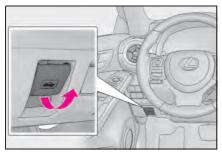
Pull the auxiliary catch lever to the left and lift the hood.
