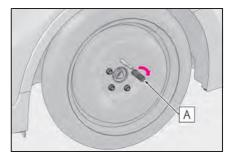
4 Remove the guide pin and loosely tighten the wheel bolt as in step 3.
