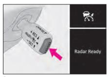
Accelerate or decelerate, with accelerator pedal operation, to the desired vehicle speed (at or above approximately 20 mph [30 km/h]) and push the lever down to set the speed.
