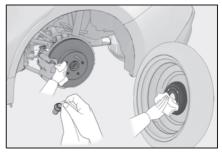
Align a wheel bolt hole on the spare tire with the guide pin, and set the spare tire on the guide pin.
