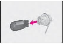
8 Install a new light bulb and then install the bulb base to the light unit
