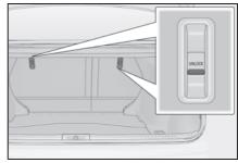
Pull the seatback lock release lever and fold the seatback down.
