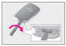
3 Remove the depleted battery.
