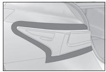
Insert a flathead screw-driver between the cover and the light unit and pry up the cover in several positions as shown in the illustration to disengage the claws (indicated by a dotted line).
