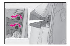
5 Pull the light unit toward the rear of the vehicle to remove it.
