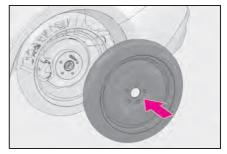
3 Loosely tighten each wheel bolt by hand or using a wheel bolt socket
