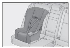
4 Run the seat belt through the child restraint system and insert the plate
