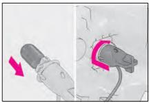
After replacing the left side bulb, install the washer fluid filler opening to its original position. 7 IS500: Install the engine compartment cover.
