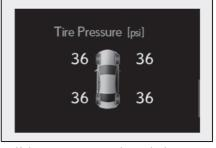
If the tire pressure drops below a predetermined level, the driver is warned by a screen display and a warning light. (→P.337)
