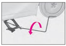
Securely tighten the wheel bolts twoor three times in the order shown in the illustration using a wheel bolt wrench.
