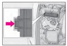
► Engine compartment: type B fuse box
