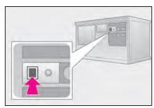
3 Press and hold the desired HomeLink<sup>®</sup> button (inside the vehicle) for 2 seconds and release it. Repeat this sequence (press/hold/release) up to 3 times to complete programming. If the garage door opener motor operates when the HomeLink<sup>®</sup> button is pressed, the garage door
