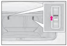
2 To disable the trunk opener, turn the main switch in the glove box off.
