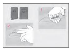
Grip the driver's door handle to unlock the door. Grip the passenger's front door handle to unlock all the doors.
